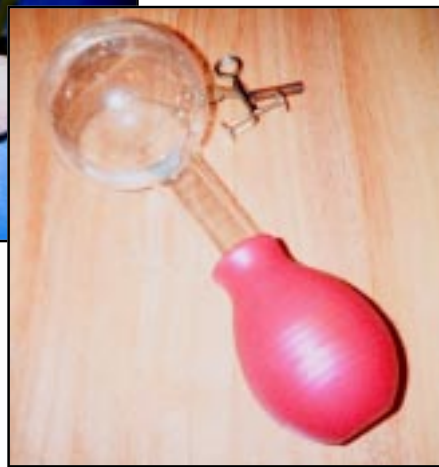
Squeezing the rubber bulb creates “high” pressure inside the apparatus. Releasing the bulb will create “low” pressure inside the apparatus, thus creating a cloud.
